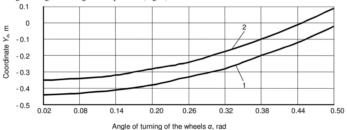
Fig. 6. Dependence of coordinate  $Y_a$  on turning angle  $\alpha$  of driven wheels of tractor with ballast on its frontal axle: 1 –  $0 \text{ kg}$ ; 2 –  $180 \text{ kg}$
