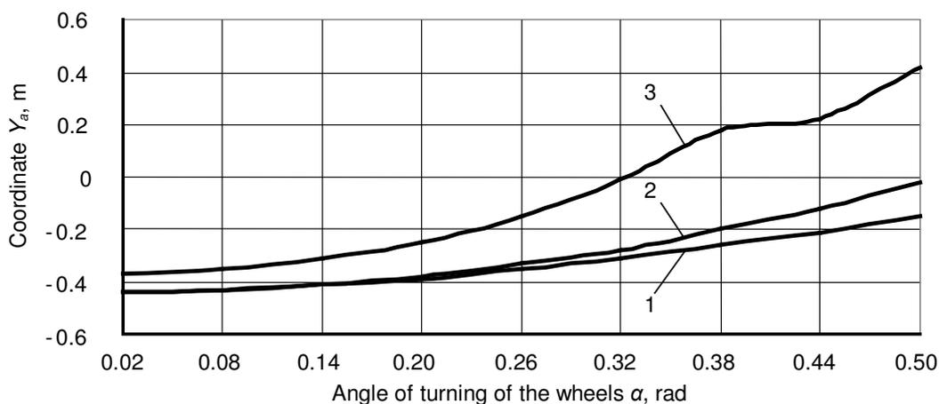
Fig. 5. Dependence of coordinate  $Y_a$  on turning angle  $\alpha$  of driven wheels of tractor at various speeds of their movement on turning strip  $V_t$ : 1 –  $1.0\text{ m}\cdot\text{s}^{-1}$ ; 2 –  $2.0\text{ m}\cdot\text{s}^{-1}$ ; 3 –  $3\text{ m}\cdot\text{s}^{-1}$
