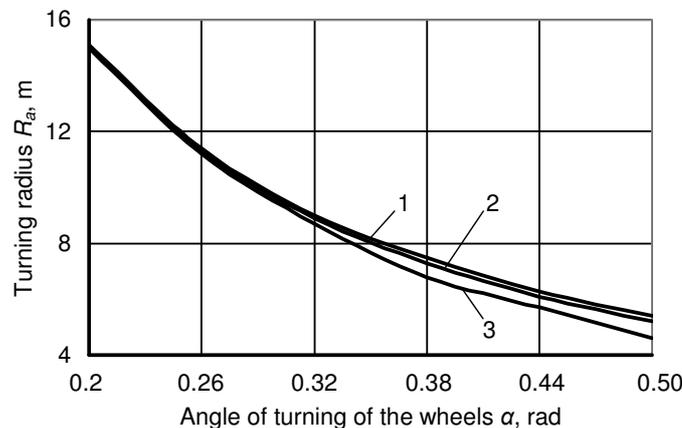
Fig. 4. Dependence of turning radius  $R_a$  of sowing aggregate on turning angle  $\alpha$  of driven wheels of tractor at various speeds of movement on turning strip  $V_t$ :
