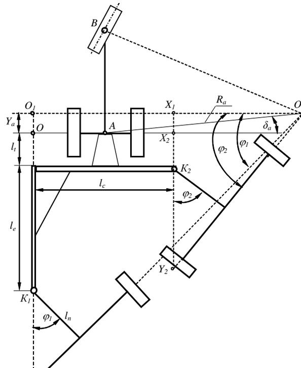
Fig. 3. Scheme for determination of turning angles of trailed seeders
